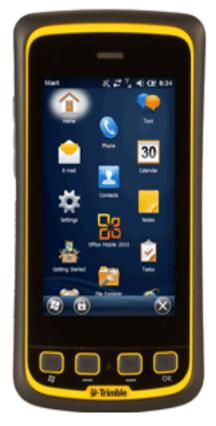
capacitive touchscreen display is sunlight-readable and brilliantly clear. Multi-touch support allows complex selections and controlled zoom to optimize the user experience with maps and detailed information. A capacitive stylus is available as an optional accessory. Users can upload and download data from the cloud using Wi-Fi or optional WWAN connections. The 8 megapixel camera can automatically include time and location data from the GPS receiver.
